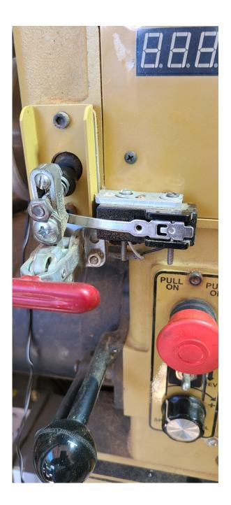
The switch is a Temco model CN101 which crosses to a Honeywell switch BZ-2RW824-A2 if the Temco is not readily available. I mounted the switch on a section of aluminum angle attached using a screw that holds the RPM plate on. The switch is wired in series to the red button start/stop switch using the normally closed contacts. The wire is routed to the back of the lathe and brought inside the headstock to make the connection. When the lever is pushed, the circuit opens and the lathe will not run.
